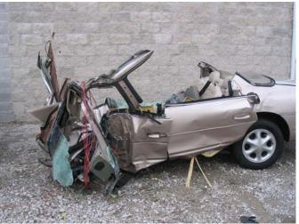
Newer automobiles are constructed with better crash protection design and materials. Some vehicles have high-strength boron steel to form a protective roll cage. This makes it more difficult for firefighters to perform vehicle rescues.
